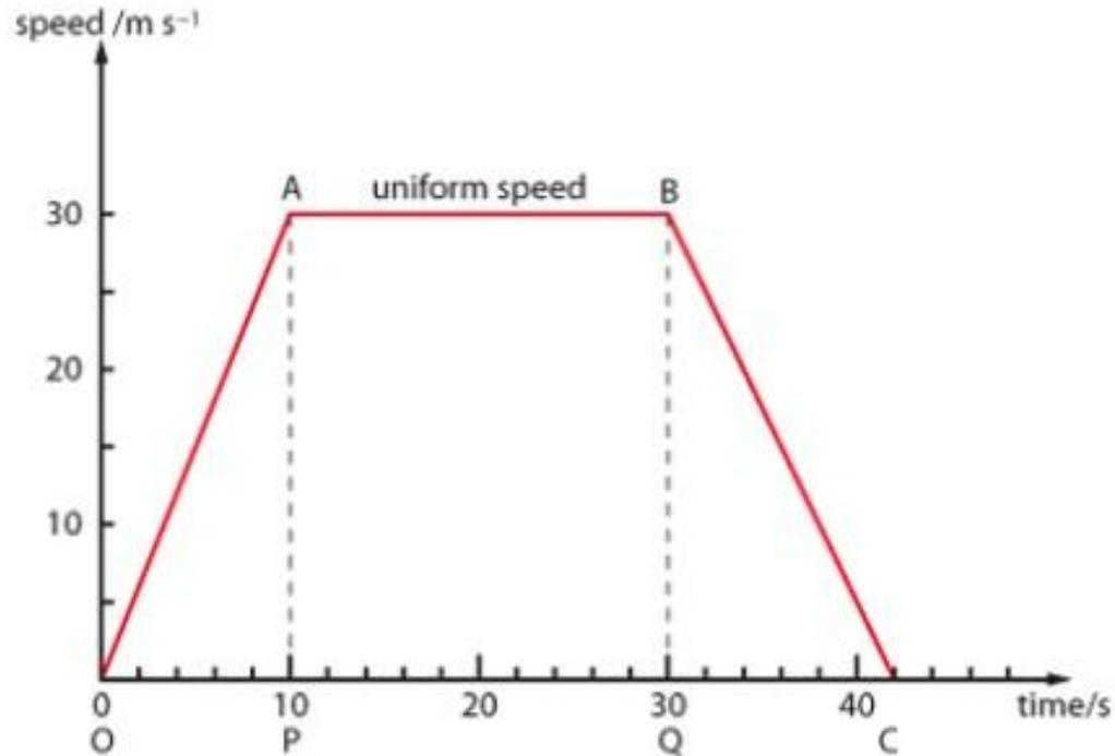
Figure 2.17 Speed-time graph of a car accelerating, moving with uniform speed and then decelerating
