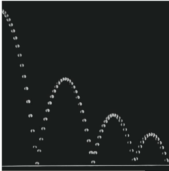
**PROJECTILE** is a body which is thrown horizontally or at an angle relative to the horizontal which follows a curved path called trajectory.
