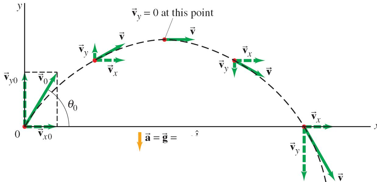
Path of a projectile fired with initial velocity  $v_0$  at angle  $\theta_0$  to the horizontal. Path is shown dashed in black, the velocity vectors are green arrows, and velocity components are dashed. The acceleration  $a = dv/dt$  is downward. That is,  $a = g$ .
