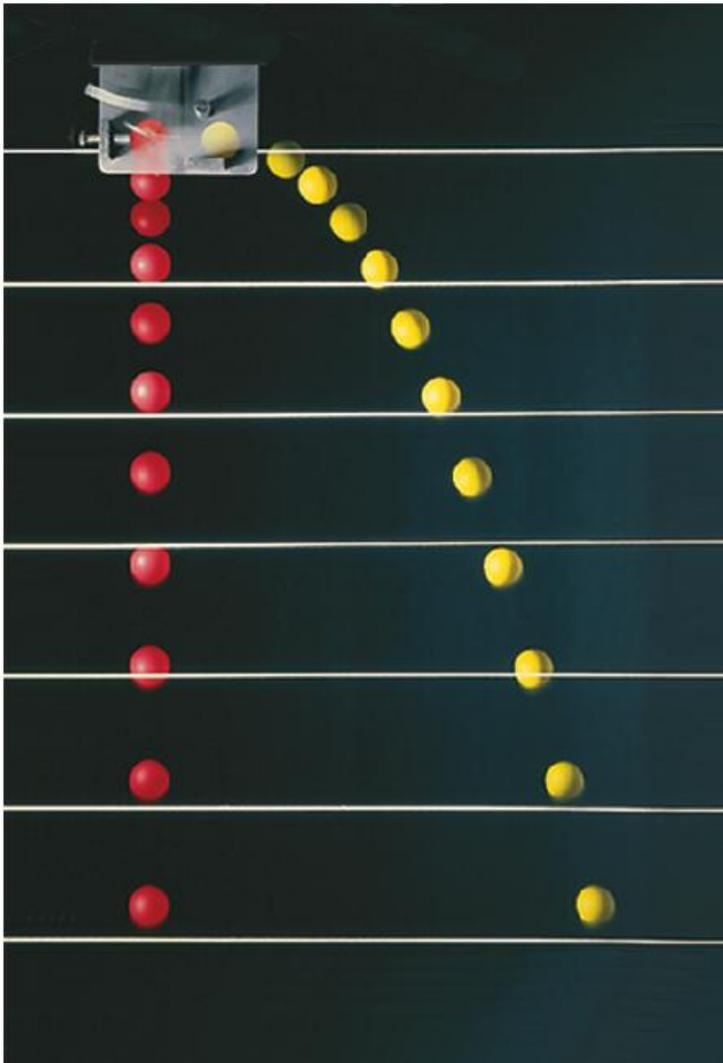
The speed in the  $x$ -direction is constant; in the  $y$ -direction the object moves with constant acceleration  $g$ .
